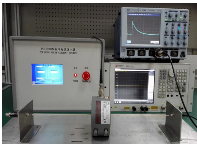
Figure 6: Test setups deployed to experimentally investigate PCI on the case of single- wire harness
