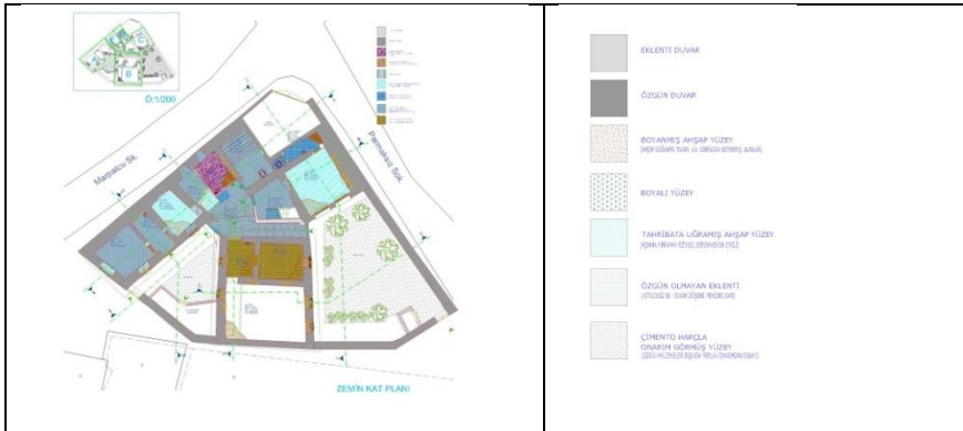
Figure 23: Example of analytical survey (The ground floor of the building in 642/1 parcel)
