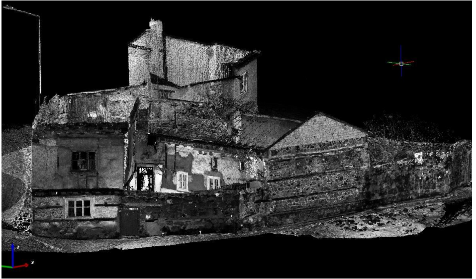
Figure 17: Terrestrial scanning studies (3D Point cloud Data)
