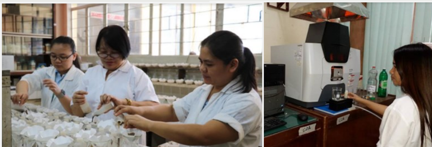
Staffs of the Regional Soils Laboratory performing (a) Zinc Assay using Atomic Absorption Spectrophotometer and (b) Extraction & Filtration of soil samples prior to analysis
