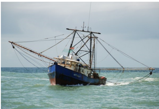
Figure 2. An outrigger trawler in the Suriname X. kroyeri trawling fleet ©Tomas Willems/ILVO
