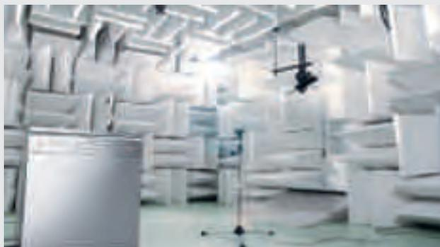
A dishwasher being monitored for sound under very specific test conditions in a laboratory before being assigned an official noise level.
