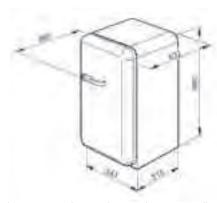
When positioning these appliances adjacent to a wall or kitchen unit a gap of 175mm must be left on the hinged side of the product to allow the door to open.
