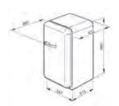
When positioning these appliances adjacent to a wall or kitchen unit a gap of 175mm must be left on the hinged side of the product to allow the door to open.
