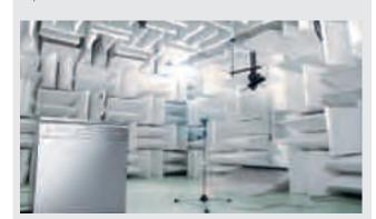
A dishwasher being monitored for sound under very specific test conditions in a laboratory before being assigned an official noise level.
