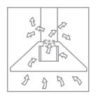
FILTER HOOD: extracts the cooking fumes and passes them through active charcoal filters, recirculating the cleaned air into the room.
