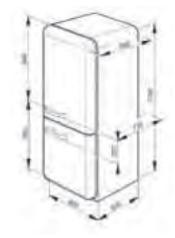
When positioning these appliances adjacent to a wall or kitchen unit a gap of 175mm must be left on the hinged side of the product to allow the door to open.
