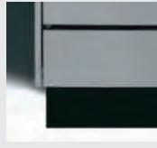
The new Concert cookers have been re-designed at the base to give custom options on the style and height. Each cooker is supplied with a set of 4 stainless steel adjustable feet and black metal plinth sections. The feet can be used alone, allowing the overall cooker height to vary between 880mm and 915mm, or if the standard 900mm height is required and the style of a sleek black plinth preferred, then the optional plinth sections can be fitted.
