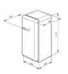
When positioning these appliances adjacent to a wall or kitchen unit a gap of 175mm must be left on the hinged side of the product to allow the door to open.
