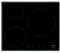
Front left: Ø 210/100mm, 1.8 kW - turbo 2.3 kW Rear left: Ø 160/100mm, 1.2 kW - turbo 2.0 kW Central right: Ø 280/100mm, 2.4 kW - turbo 3.6 kW
