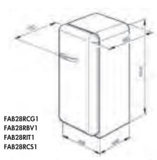
When positioning these appliances adjacent to a wall or kitchen unit a gap of 175mm must be left on the hinged side of the product to allow the door to open.
