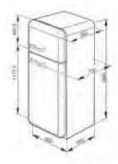
When positioning these appliances adjacent to a wall or kitchen unit a gap of 175mm must be left on the hinged side of the product to allow the door to open.
