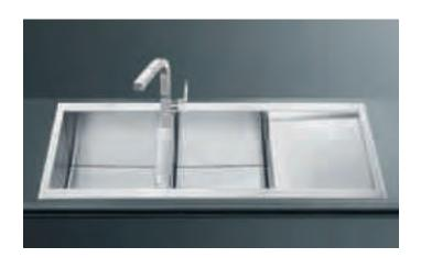
Linear range, reversible sink with pop-up command Double bowls, low profile sink, st/steel 1mm thick Brushed st/steel, plain drainer, minimal design 2 bowls 350 x 400mm Bowl depth 210mm 3mm high on kitchen top 3,5" strainers
