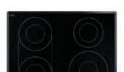
Front left: Ø 180mm, 2.0 - turbo 2.8 kW Rear left: Ø 180mm, 2.0 kW - turbo 2.8 kW Rear right: Ø 160mm, 1.4 kW - turbo 2.0 kW Front right: Ø 230mm, 2.0 kW - turbo 3.1 kW
