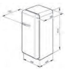
When positioning these appliances adjacent to a wall or kitchen unit a gap of 175mm must be left on the hinged side of the product to allow the door to open.
