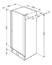
NB: If the cooler is built-in a space of at least 5cm must be left behind and above the appliance.
