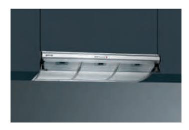
1 High performance motor, 125W 3 speeds 2 x40W lamps 3 metal grease filter Internal re-circulation possible Vent outlet Ø 130mm Nominal power 205W
