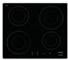
Front left: Ø 210/100mm, 1.8 kW - turbo 2.3 kW Rear left: Ø 180/100mm, 1.6 kW - turbo 2.3 kW Rear right: Ø 210/100mm, 1.8 kW - turbo 2.3 kW Front right: Ø 160/100mm, 1.2 kW - turbo 2.0 kW
