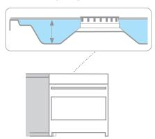
In contrast to many traditional cookers, all Smeg hob tops have an **anti-overflow feature**, with the 90cm models capable of holding 4.5 litres. This special feature avoids spills of liquid thus protecting the kitchen furniture on either side.
