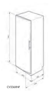
New rounded aesthetic Reversible door Total gross capacity 231 litres No-Frost Adjustable thermostat Fast freezing function ECO function
