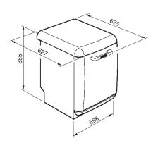
NB: This dishwasher will not fit under a standard worktop. Please check measurements carefully and choose the built-in version if there is insufficient height.
