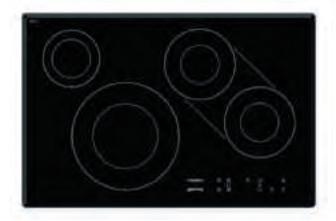
Front centre: Ø 280mm, 2.6 kW - turbo 3.7 kW Front left: Ø 145mm, 1.4 kW - turbo 2.2 kW Rear right: Ø 180mm, 1.8 kW - turbo 3.0 kW Front right: Ø 180mm, 1.8 kW - turbo 3.0 kW
