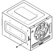
2. Pull out the Rear Bracket (as shown below:)
