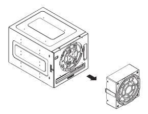
(\*Note: For the SC-942 Chassis, the CSE-M35 Rear Exhaust Fan should not be used. Instead, the hot-swappable 120mm Chassis Fans included with the SC-942 Chassis should be connected to the Backplane of the CSE-M35S/CSE-M35T1 Mobile Rack.)
