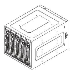
2. Swing the handle outward and pull out the unit (as shown below:)
