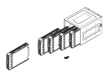
3. Mount a drive in a carrier (as shown below:)
