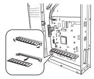
5 Insert the new DIMM straight down into the DIMM connector until the latches snap into the locked position.
