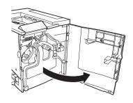
3 Insert the thumb and index finger of vour hand into the two holes in the front of the toner cartridge, and then pull the cartridge straight out about 6" (152 mm).
