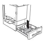
$oldsymbol{3}$  Load the paper face-up, short edge (or letterhead) toward the right of the tray. Often, an arrow on the media package label indicates the printing-side of the media. Do not overfill the tray.
