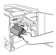
**4** Support the middle of the cartridge with your left hand, and then pull out the cartridge.
