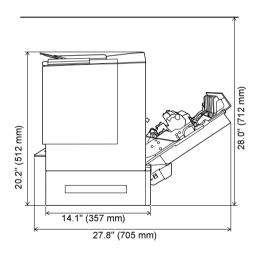
If you have added the optional lower feeder unit, the printer's height will increase by approximately 5" (125.5 mm).
