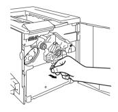
5 Wipe the surface of the laser lens cover with a soft, dry cloth.
