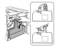
Place the removed waste toner bottle, with the openings facing up, on a stable surface (not the printer).
