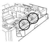
10 With the right door still open, place the printer on the lower feeder unit.
