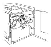
2 Grasp the release lever on the OPC drum cartridge, and then pull the cartridge straight out about 6 inches (152 mm).
