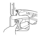
2 Remove the cover from the right side of the printer. Use a Phillips screwdriver to remove the two screws securing the right cover.
