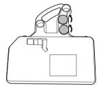
4 Secure the two caps onto the two holes by turning them clockwise.
