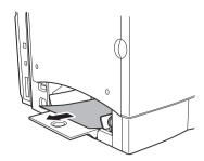
3 Fan the removed media to prevent static buildup and even up the front edges.
