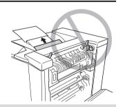
If it is difficult to remove the jammed media, turn the misfeed-clearing dial counterclockwise to feed the media downward.
