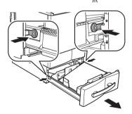
2 Carefully remove the jammed media in the direction shown on the illustration and dispose of it.
