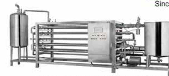
Pasteurizer for beverage and milk.
