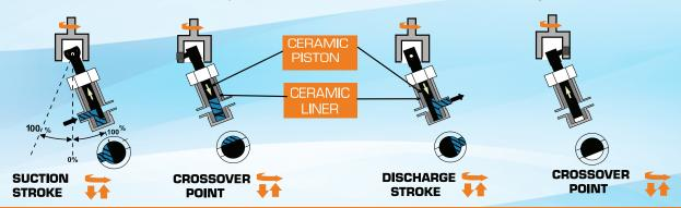
reciprocates. As the piston is pulled back and the piston flat opens to the inlet port, suction is created and fluid fills the pump chamber. As the piston reaches the highest point in the reciprocation cycle, the pump chamber is now at its maximum volume capacity. Continuing the rotation, the inlet port is then sealed
