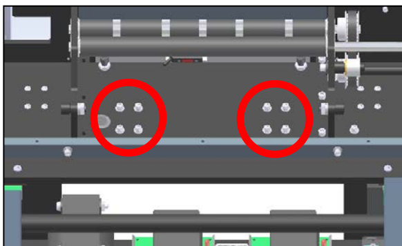
Figure 3-316. Heater Block Mounting Screws Note: Viewed from Rear; Cradle Removed for Clarity
