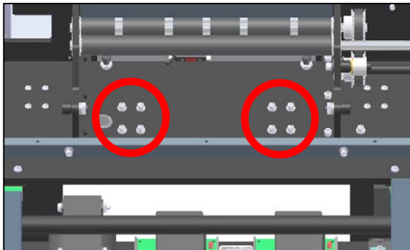
Figure 3-340. Heater Block Mounting Screws Note: Viewed from Rear; Cradle Removed for Clarity
