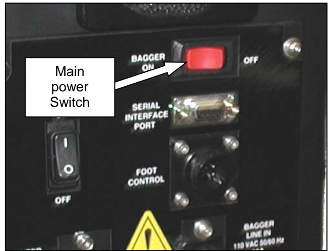
Figure 3-53. Main Red Switch location
