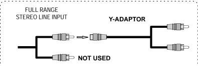
Note: You can use the Radio/CD designated mono line output or a full range stereo line output. For full range stereo line output, you will need an optional "Y-Adaptor" as shown.
