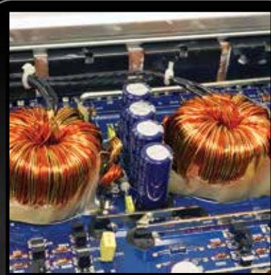
Twin turbo power supply torroids in a PWM MOSFET power supply design
