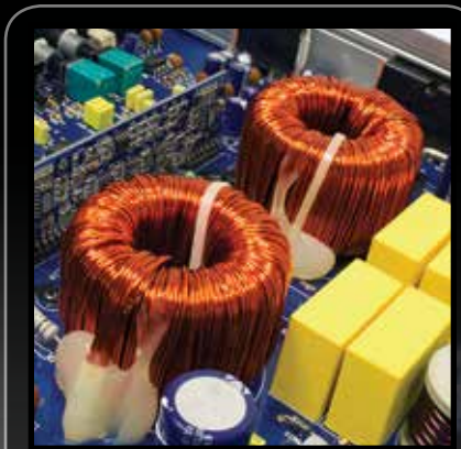
SPC Simpatico Coil Design Pulse Width Modulated power supply
