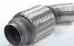
Repair Pipe Bellow for BMW · HJS-No. 83 00 8325 Dimensions: Ø 70 x 279 mm
