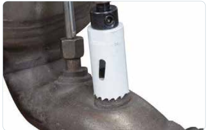
4. Cut out temperature sensor connection using a \varnothing 25 mm hole saw without centering bit. ! Special precautions must be made, that no debris remains in the filter housing.
