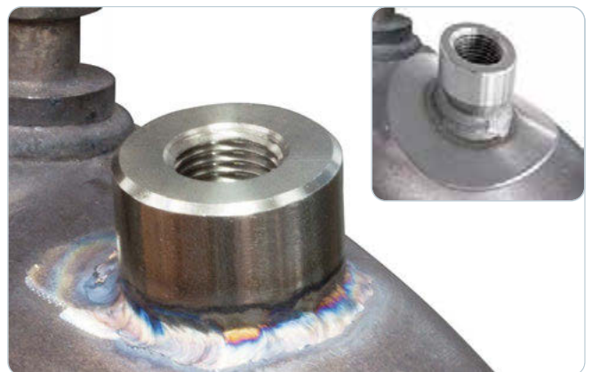
6. Insert HJS repair connector and weld in.
