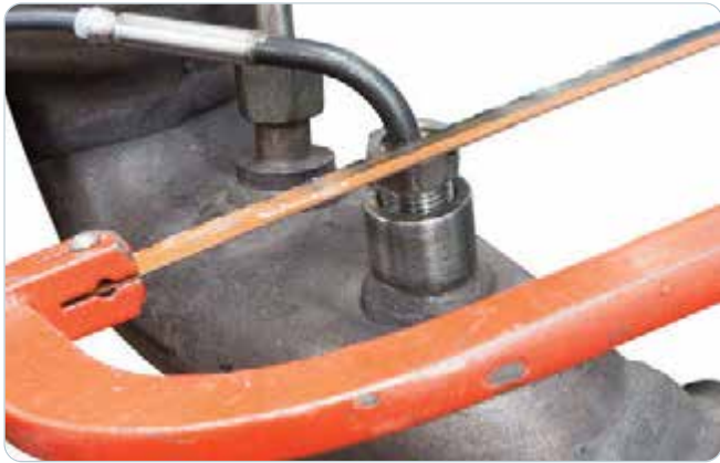
1. Remove DPF® according to manufacturer's instructions. Cut off defective Temperature sensor (sensor tube).
