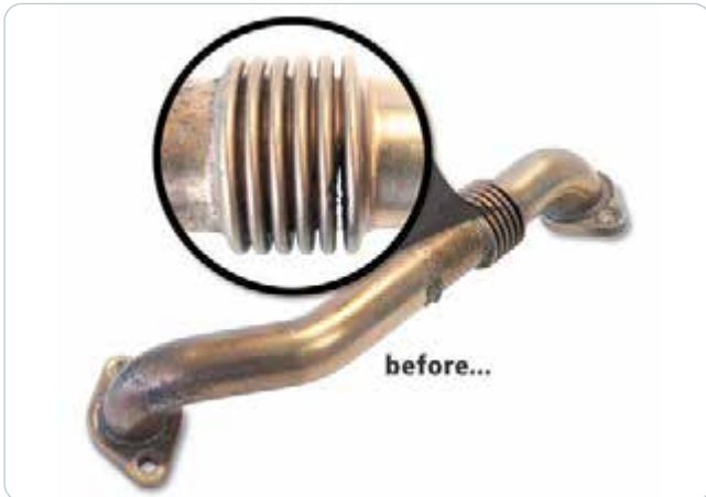
Bellow pipe cracked
