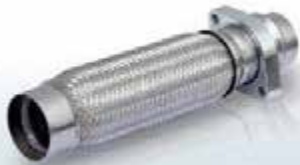
Bellow for BMW · HJS-No. 83 00 8314 (right-hand) Dimensions: Flange Length = 275 mm
