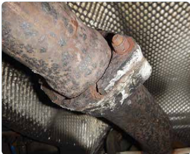
Picture shows flange connection from a BMW 530 i
