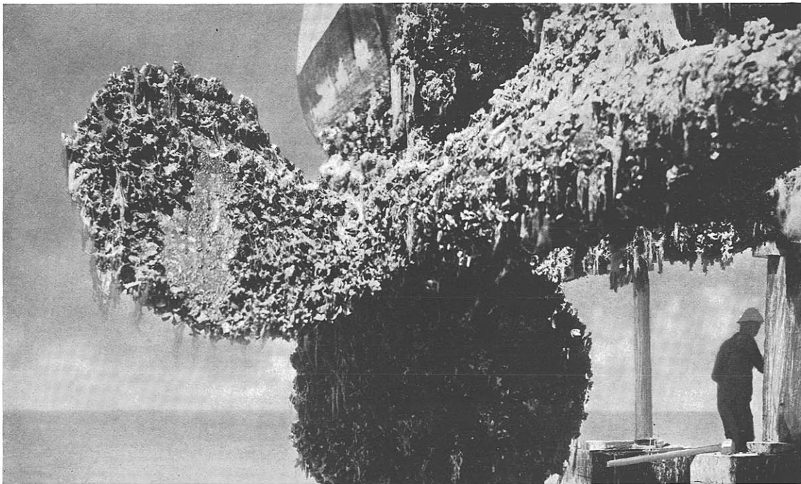
Heavy accumulations of barnacles and other marine organisms fouling a ship's propeller. After Visscher. Courtesy of the Bureau of Fisheries
