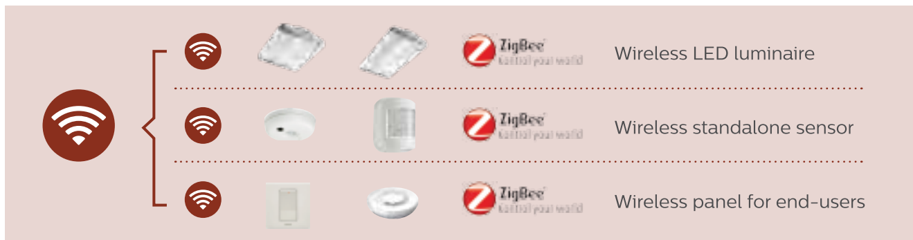
Master luminaire connected to slave luminaires, standalone sensor and wireless panels
