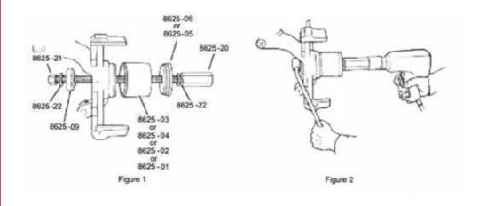
Important: Assemble the adapter with the flat side toward the housing, and the small diameter pilot on the side away from the housing.
