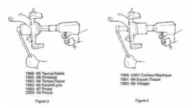
4. Lightly lubricate the new bearing, and position it for installation with the tool components assembled as shown.
