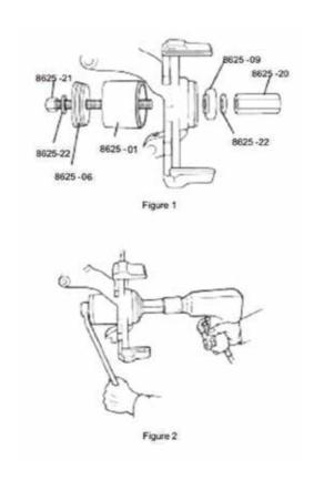
Important: Assemble the adapter with the flat side toward the housing, and the small diameter pilot on the side away from the housing.
