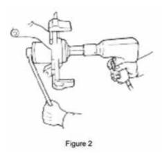
Important: Assemble the adapter with the flat side toward the housing, and the small diameter pilot on the side away from the housing.
