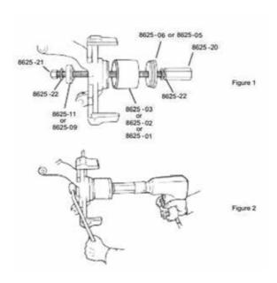
Important: Assemble the adapter with the flat side toward the housing, and the small diameter pilot on the side away from the housing.
