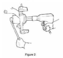
Important: Assemble the adapter with the flat side toward the housing, and the small diameter pilot on the side away from the housing.
