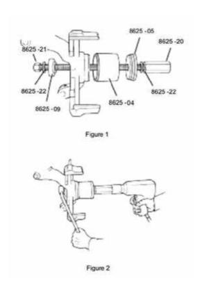
Important: Assemble the adapter with the flat side toward the housing, and the small diameter pilot on the side away from the housing.
