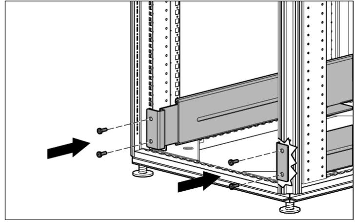
5. Tighten the wing nuts or hex nuts.
