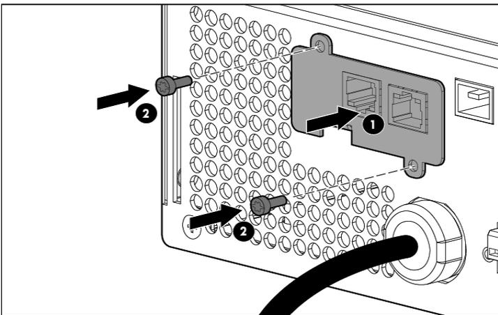
3. Secure the UPS Network Module using the two screws you removed in step 1.
