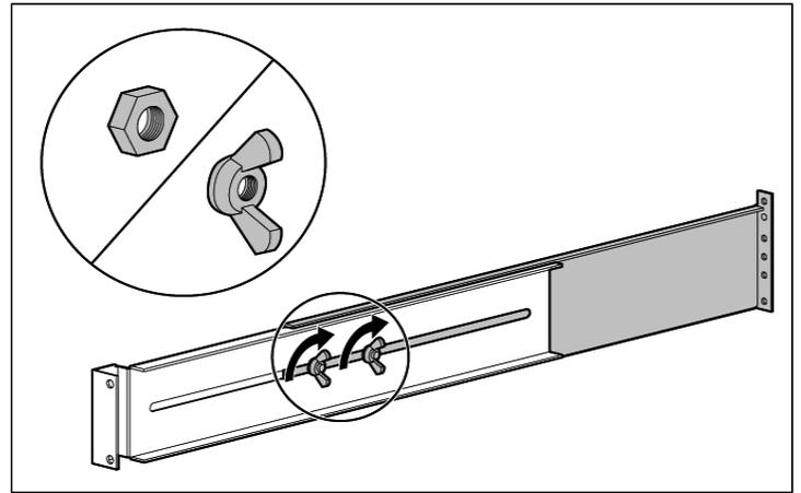
6. Install the rear stabilization bracket using wing nuts. Wait until the unit is installed and the brackets are adjusted before tightening the nuts.
