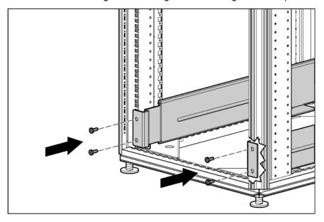
Tighten the wing nuts or hex nuts.
