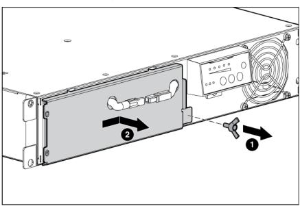
Remove the UPS battery modules.
