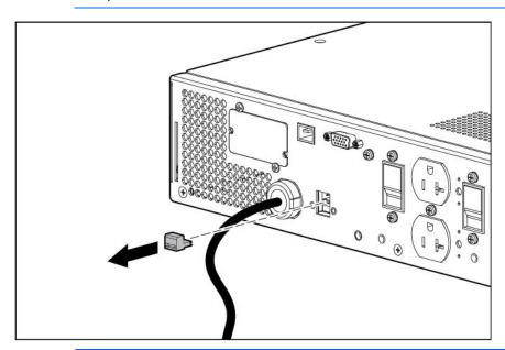
**NOTE:** Wire the connector block using stranded, nonshielded wire (AWG #22 - #18, or equivalent).
