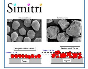
Simitri Polymerized Toner adheres better to the media surface as a result, prints are more durable, with images and text that don t smear or fade.
