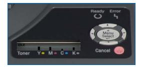
The magicolor 2530 DL has a user-friendly control panel that guides you through such things as supply changes and print job setup. The magicolor 2530 DL has two LEDs (Ready and Error) that indicate printer status.
