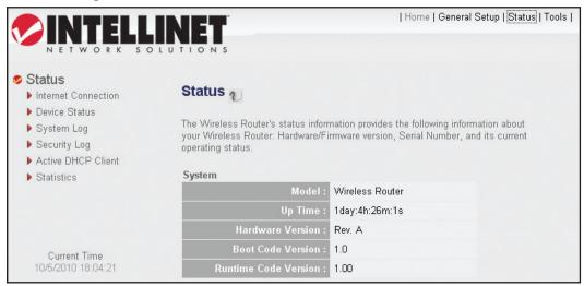
In case you experience technical difficulties with the router and need to contact technical support, you should write down the Boot Code Version and Runtime Code Version shown on your screen (which may vary from the example shown here). It is very likely that you would be asked to provide these numbers by the technical support representative.
