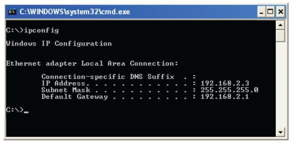
*NOTE:* If the IP address of the gateway is not displayed, or if the address begins with 169, recheck the network connection between your computer and the router, and re-check each step of the network setup procedure.
