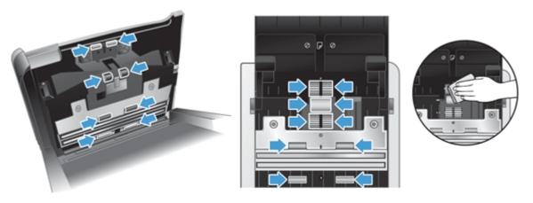
Wipe the rollers from the top down, rotating the rollers a full 360 degrees to ensure that you wipe the complete surface.
