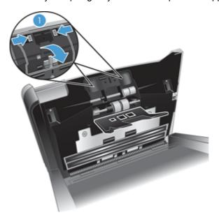
5. Using the paper path cleaning cloth that came with your scanner (or a clean, lint-free cloth moistened with isopropyl alcohol), wipe the feed rollers on both sides of the open hatch.
