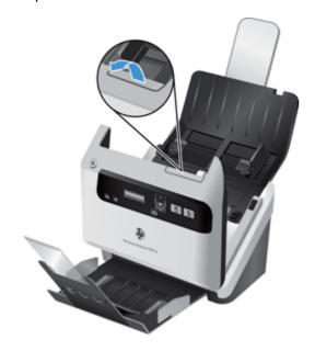
On the rear of the open document feeder, raise the feed roller covers to expose the upper feed rollers.
