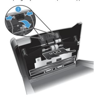
5. Using an HP paper path cleaning cloth or a clean, lint-free cloth moistened with isopropyl alcohol, wipe the feed rollers on both sides of the open hatch.
