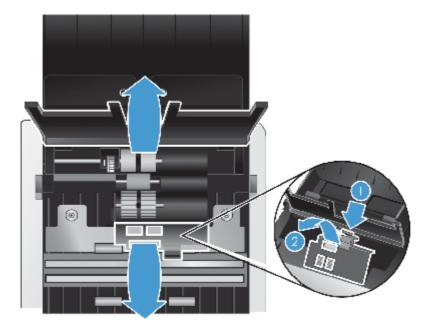
4. On the front of the open document feeder hatch, squeeze in on the tabs on the roller door assembly and pull gently forward to expose the upper feed rollers.
