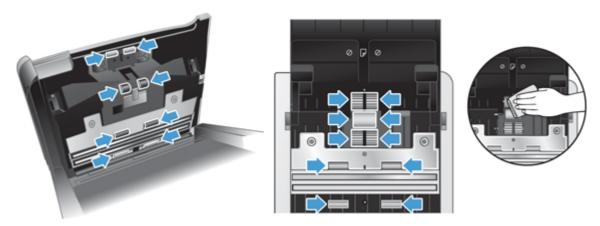
Wipe the rollers from the top down, rotating the rollers a full 360 degrees to ensure that you wipe the complete surface.
