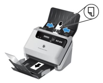
2. Adjust the paper guides to center the cards, making sure the paper guides touch the edges of the cards.
