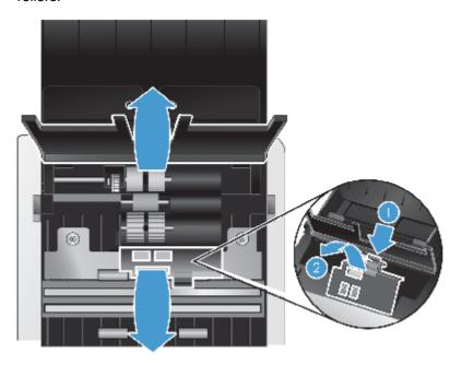
On the front of the open document feeder, squeeze in on the tabs on the roller door assembly and pull gently forward to expose the upper feed rollers.
