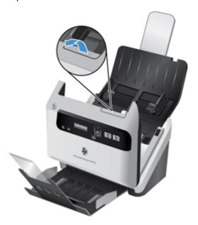
On the rear of the open document feeder hatch, raise the feed roller covers to expose the upper feed rollers.
