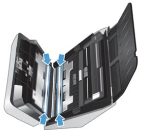
CAUTION: Use only glass cleaner to clean the scanning strips. Avoid cleaners that contain abrasives, acetone, benzene, and carbon tetrachloride, all of which can damage the scanning strips. Avoid isopropyl alcohol because it can leave streaks on the scanning strips.
