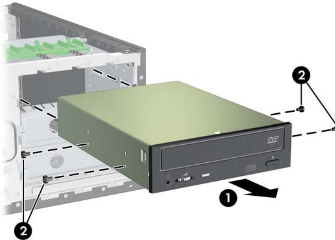
Figure 5-18 Removing the optical drive screws
