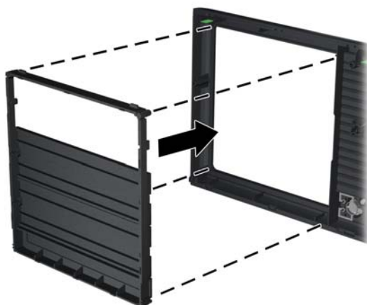
Figure 5-47 Installing the ODD bay filler panel
