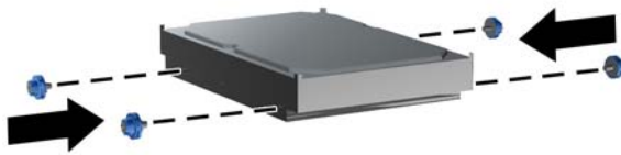
Figure 5-37 Installing the grommet screws
