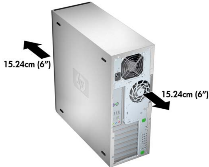
Figure 1-5 Proper computer ventilation
