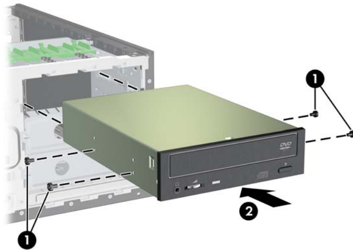
Figure 5-19 Installing the optical drive
