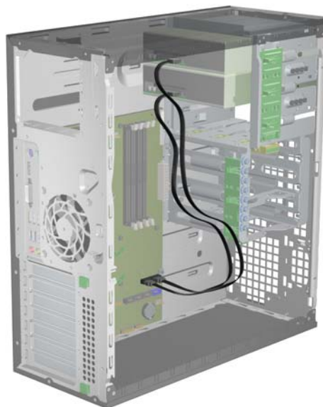
Figure 5-15 Connecting multiple power and data cables
