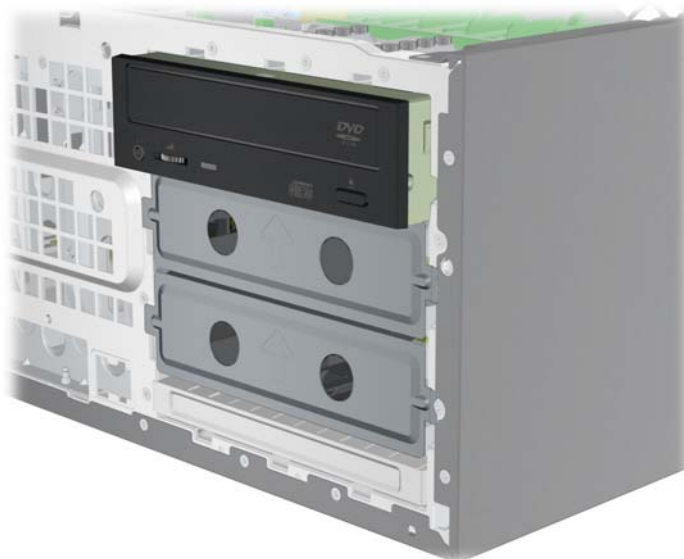
Figure 5-49 Reinstalling the optical drive
