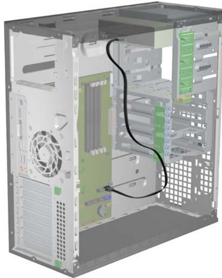
Figure 5-15 Connecting multiple power and data cables
