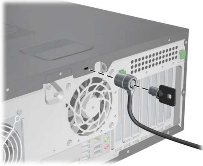
Figure 5-2 Removing the cable lock
