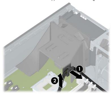
5. Remove the airflow guide by pulling it straight up and out of the chassis, as shown in the following figure. (The processor heatsink is not shown.)
