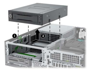
8. If you are replacing the DX115 unit, remove and retain the four M3 x 5mm screws (black) from the lower four mounting holes of the DX115 case, and then transfer the screws to the new unit. (You can also store the screws in the chassis. See <u>Locating extra guide screws on page 72</u> for screw locations.)
