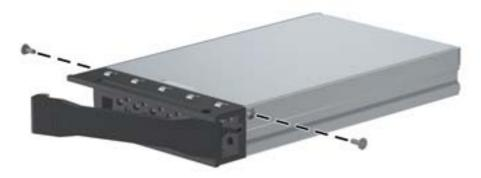
11. Install the carrier in the drive case:
