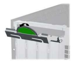
5. Push the retention latch (1), and then carefully lift the card from the chassis (2).
