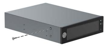
4. Install four (supplied) M3 x 5mm screws (black) in the lower four mounting holes of the DX115 case. (See <u>Locating extra guide screws on page 72</u> for screw locations.)
