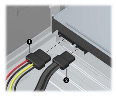
7. Press down on the green release latch next to the hard drive (1). While holding the latch down, slide the drive forward until it stops, then lift the drive up and out of the bay (2).
