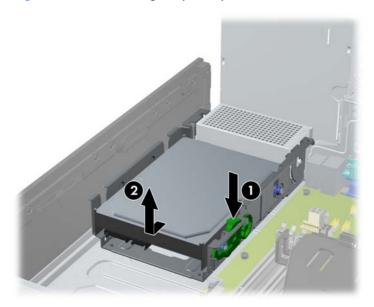
**8.** To install a new hard drive, move the silver and blue isolation mounting guide screws from the old hard drive to the new hard drive.
