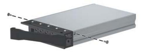
**b.** Remove the carrier cover by raising the front end of the cover (1) and pulling it away from the slot in the rear of the carrier (2).
