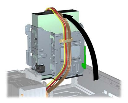
5. Rotate the power supply to its upright position. The hard drive is located beneath the power supply.
