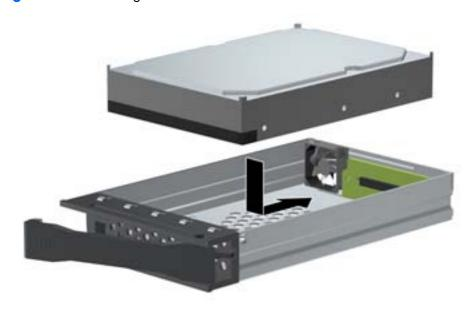
**f.** Replace the cover by aligning the tab on the rear of the cover with the slot on the rear of the carrier (1) and then rotating the front of the cover onto the carrier (2).
