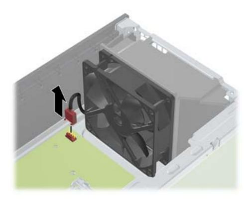
7. Remove the fan assembly by pushing in on the four release tabs on the front of the chassis (1), and then sliding the fan assembly into the chassis until you can lift it out.
