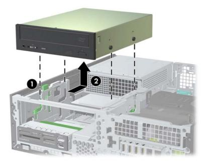
8. If you are replacing the drive, transfer the four guide screws from the old drive to the new one.
