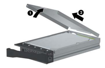
**c.** Remove the drive by sliding it toward the front of the carrier until it disengages from the carrier adapter and then lifting the drive out of the carrier.
