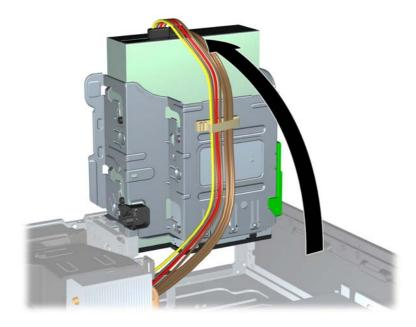
5. Disconnect the power cable (1) and data cable (2) from the rear of the optical drive.
