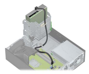
9. If necessary, route the data cable through the cable guides. There are two cable guides that keep the data cable from being pinched by the drive cage when raising or lowering it. One is located on the bottom side of the drive cage. The other is located on the chassis frame under the drive
