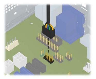
Figure 5-20 Disconnecting the Media Card Reader 1394 Cable
