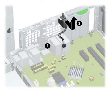
4. Slide the sensor back in its slot, push the sensor down, and then remove it from the chassis (2).
