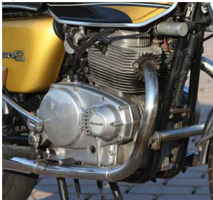
The 643cc air-cooled parallel twin makes 50 horsepower (left). The sweet sounding Lafranconi mufflers (right).
