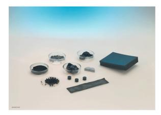
Figure 6: Typical Vacuum Energy polymer hydrogen getters. [23]
