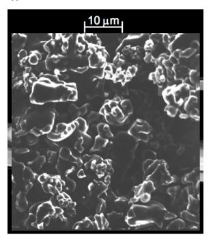
Figure 4: Sintered porous getter structure of a Zr alloy. [17]
