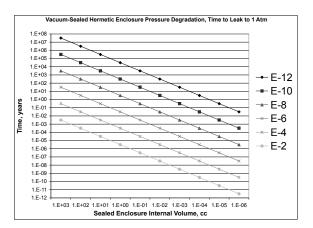
Figure 2: Time to reach 1 atm from a vacuum for various leak rates and device volumes. [3]
