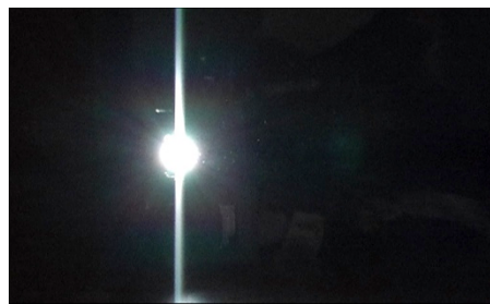
Figure 38 - Pixel saturation of a CCD camera [43] [44]
