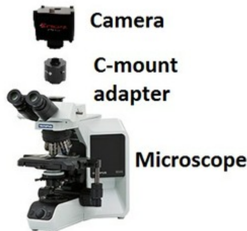
Figure 32 - Camera c-mount incorporating a relay lens [36]
