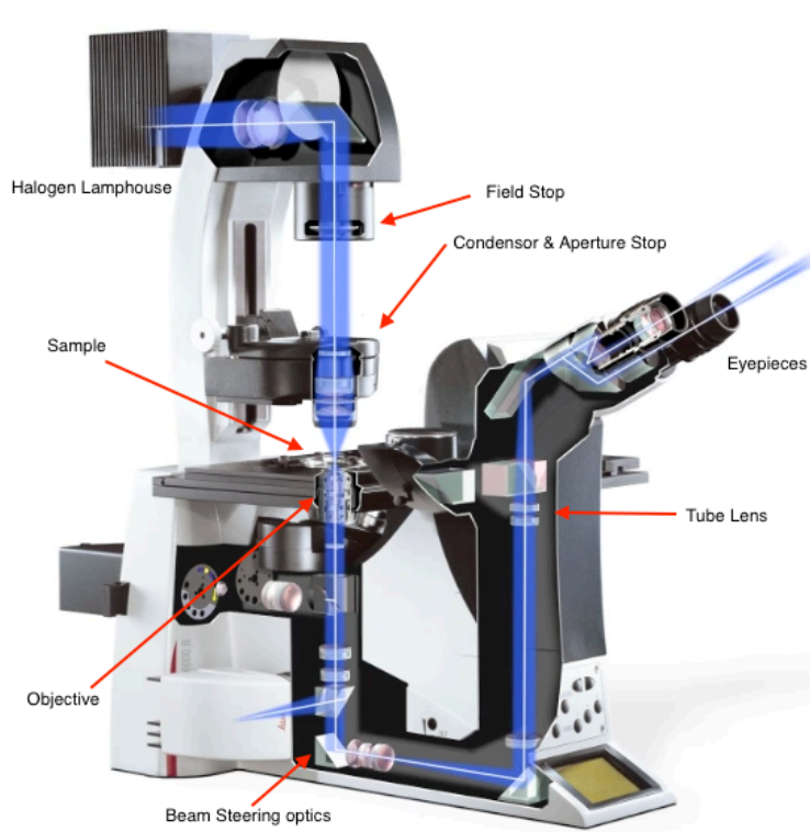
Figure 30 - Inverted microscope lightpaths [34]
