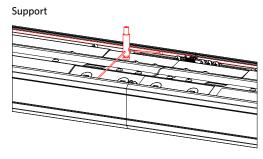
Proper allows the installer the ability to avoid obstructions with up to 24" of travel between fixtures, and 12" of travel at the beginning and end of the run. If adjusting the feed location, please ensure that you have 12" of extra cord length to accommodate your drop distance.
