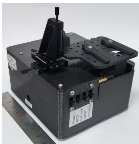
Fig. 1 Photo of the palm-top microchip electrophoresis device
