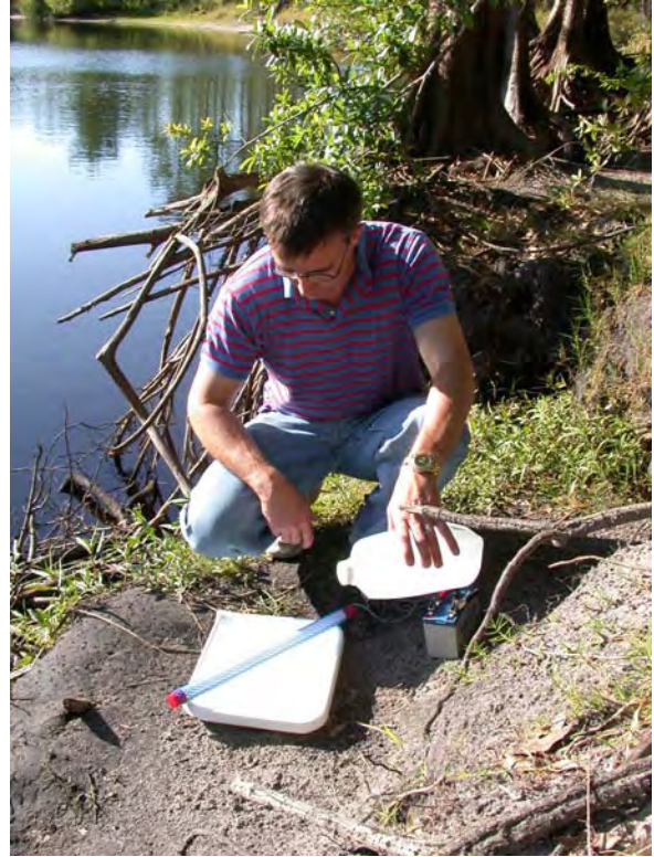
Figure 2. Light-trapping method used to capture adult caddisflies in field survey.
