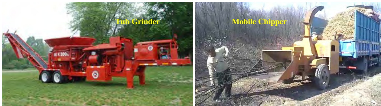
Figure 1 Examples of portable grinding and chipping equipment for processing green wastes.
