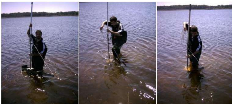
Figure 6: Phases with which a manual box corer is used (Sangiorgio et al., 2009).
