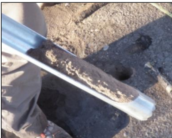
Figure 2. 8: Soil corer with 10 cm of soil. Six cores were collected on each plot.
