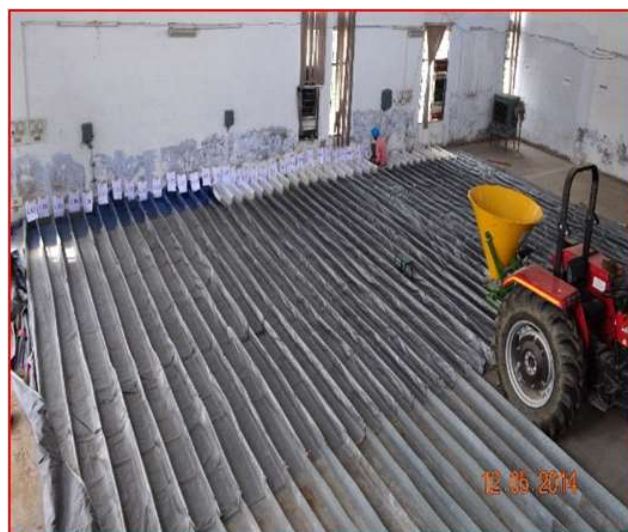
Fig. 2. Setup for evaluation of fertilizer broadcaster
