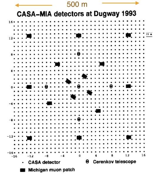
1089 detectors with 15 m spacing covering an area of  $\sim$  500 m  $\times$  500 m
