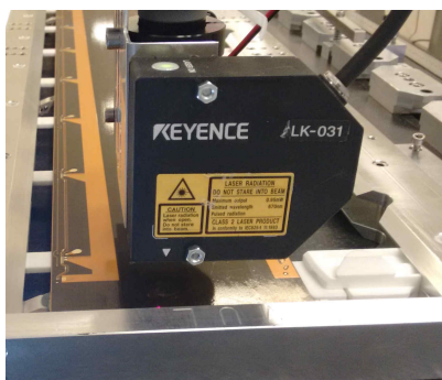
(a) Laser range finder above a prototype stave. The red measurement dot is visible.
