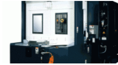
• Makino A66 FMS with connected DM w/17 pallet system. (660*660*880mm work area) 2pc
