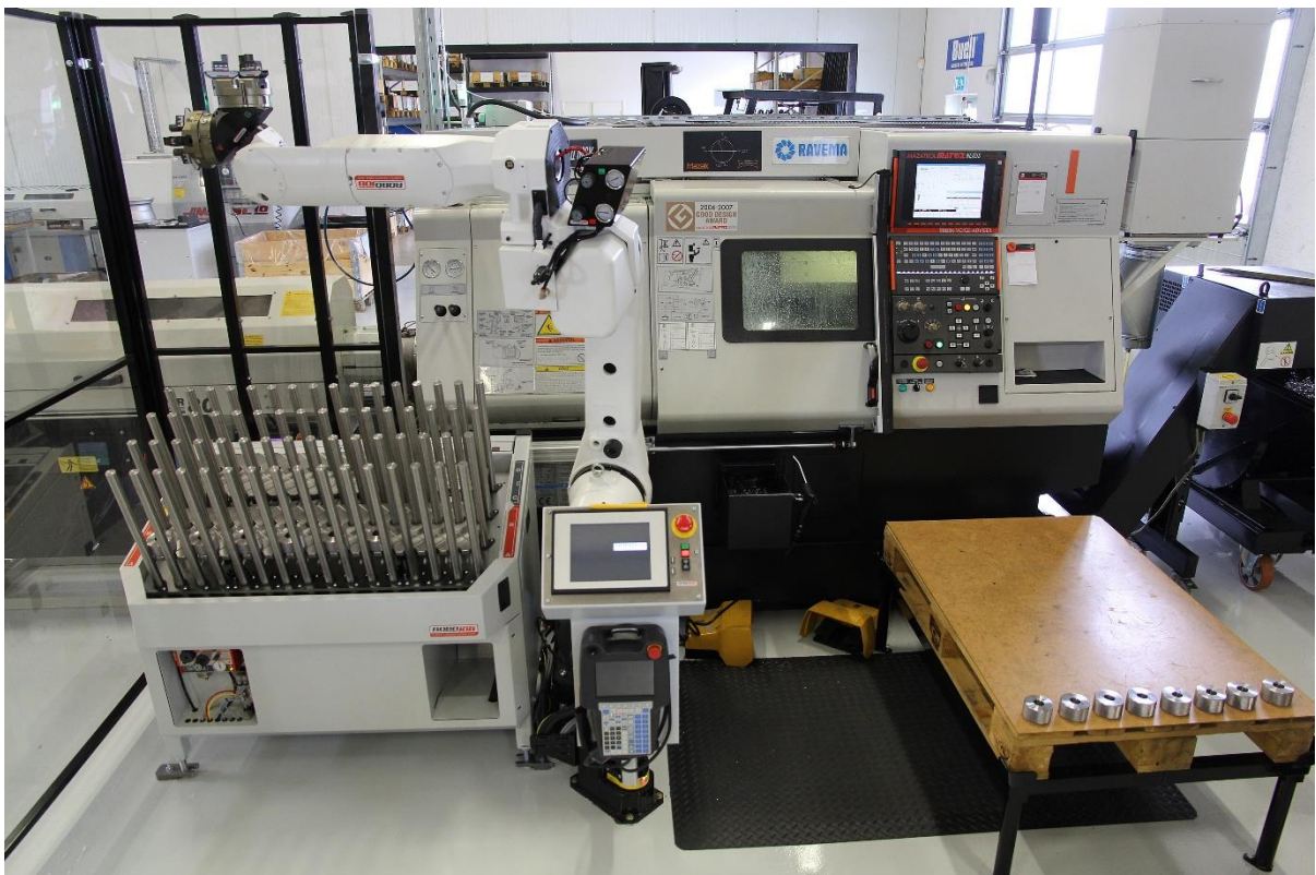
Mazak 250 MSY- Turnig/milling-Barfeeder & Robot
