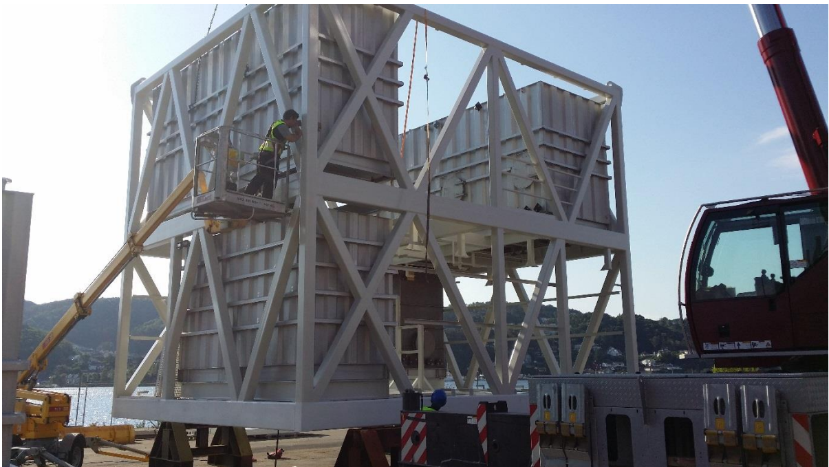
Mariner Chemical Injection Skid. Carbon steel frame, AISI 316L, 22Cr Duplex, and Titanium vessels. Aluminium railings and grating.
