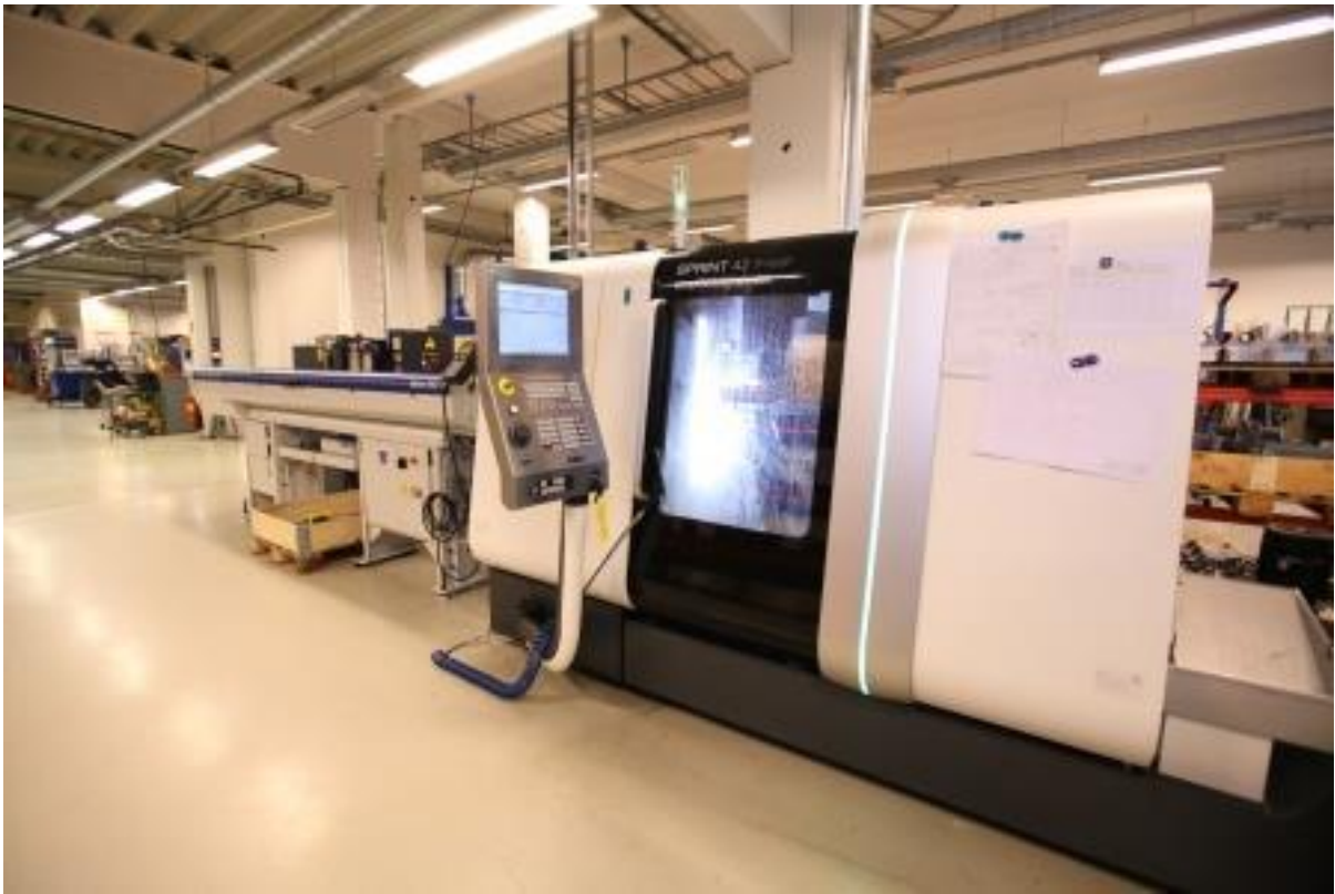
Gildemeister turning machine with bar feeder for larger series
