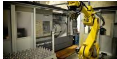
Okuma MU-VA500-L. Full 5-axis milling machine with turning function. Connected robot and 3 pallet system. (500*500*500mm work area)
