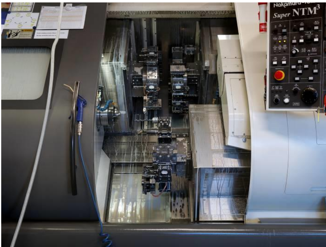
Nakamura lathe with 3 turrets for optimal efficiency, stability and quality when machining demanding materials.
