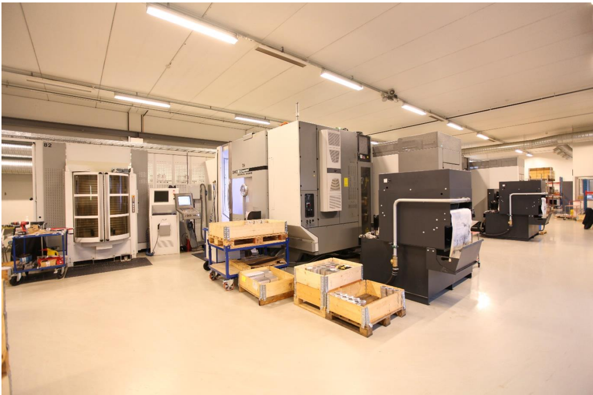
2 x Deckel Maho 80 (each with 240 tools) attached to 24 pallet Fastems systems. High efficiency for production in different sorts of aluminum, and other metals.
