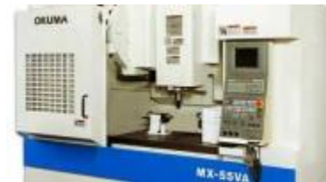
Okuma MX55VA 5-axis (550*550*550mm work area).
