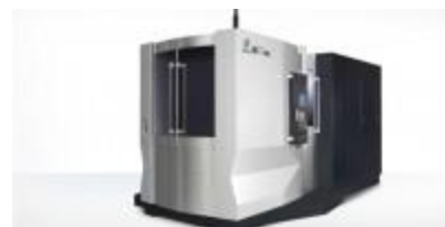
Makino A 61 NX w/2 pallet system. (610*610*880mm work area)
