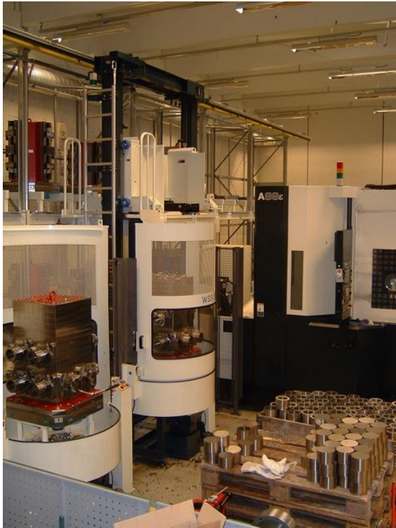
2 x Makino FMS A88E with 20 pallets system with robot.
