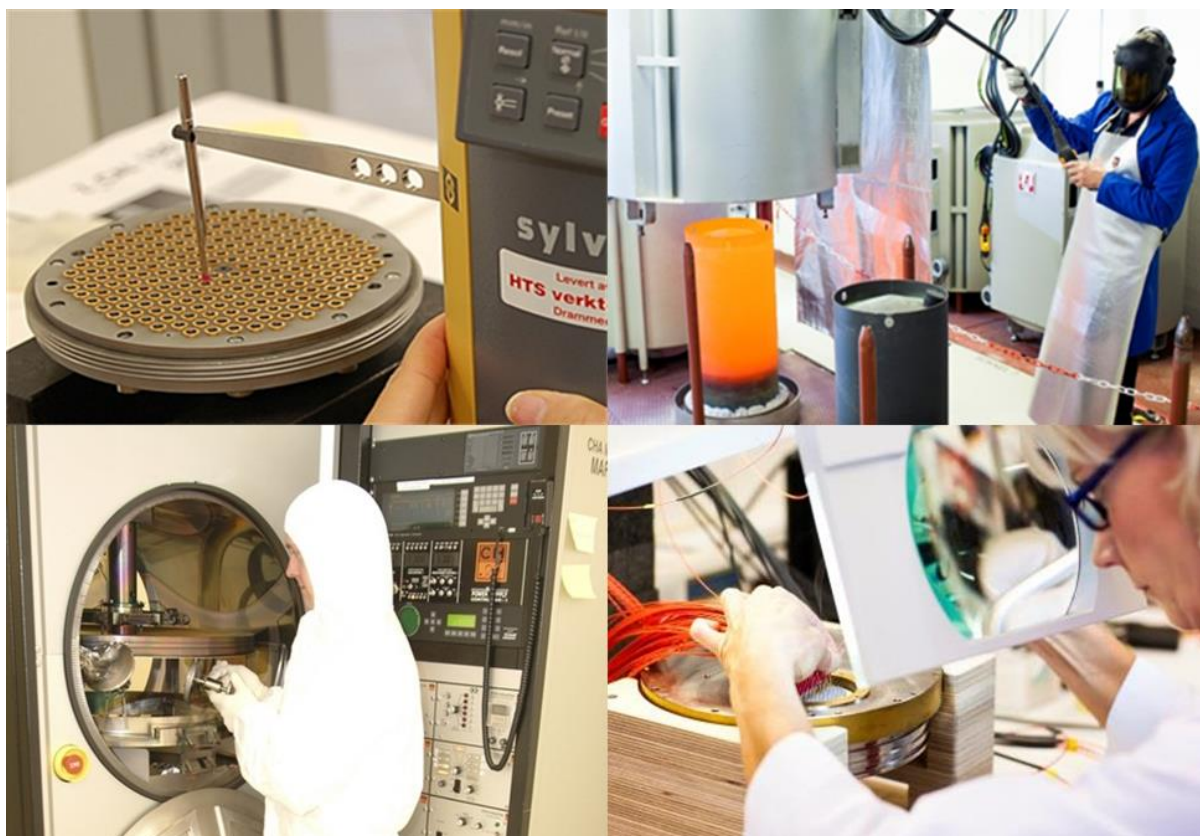
High temperature glass sealing, Additional PVD options, assembly, wiring, soldering
