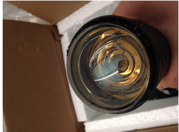
(b) A fully cleaned PMT, after some intensive scraping with a razor blade.
