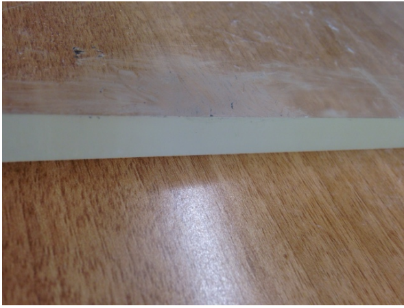
FIG. 15: Adhesive left after taping the sides of the scintillator to prevent scratching by the sandpaper used to polish them.
