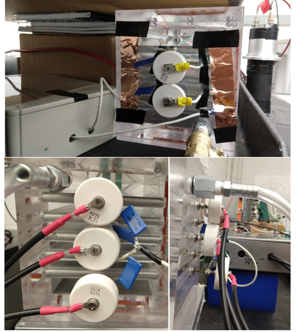
FIG. 32: Evolution of the back face of the box with prototyped capacitor-adaptor constructions from an early design with copper tape buses to threaded capacitors (top) to a more secure construction using coaxial cables (bottom, left and right).
