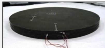
Interlayer temperature sensors installed for a flat disk test specimen
