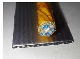
Figure 4. FFC cable versus standard SpW cables
