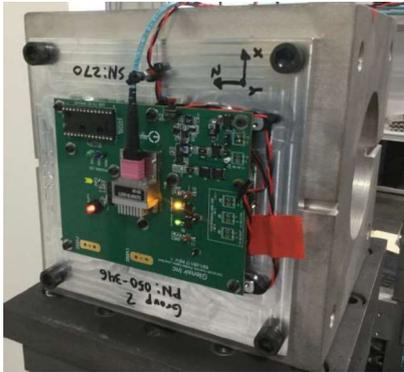
Fig. 9. Parallel optical transceiver on evaluation board, mounted on vibration and shock test fixture for operational loop-back test at 10 Gbps while undergoing shock and/or vibration exposure.
