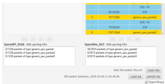
Fig. 10. Portion of Sniffer GUI visualization of XML tab where 56 packets have been identified by their XML structure.
