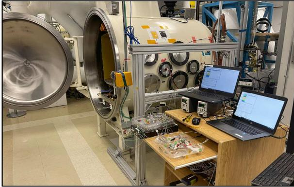
Figure 11. TVAC Testing Chamber and Test Station
