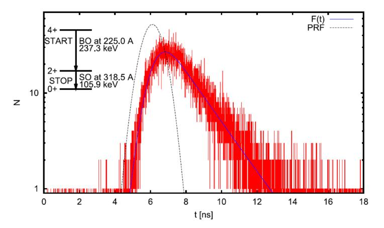
Gaussian-exponential convolution to account for timing resolution
