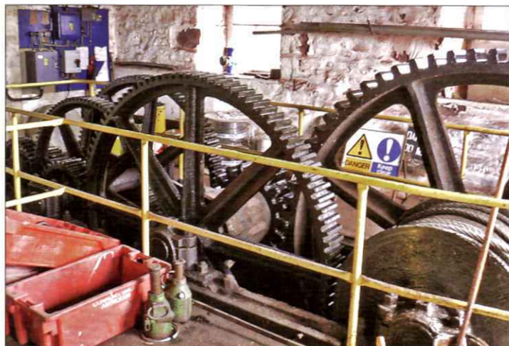
AR6: Arbroath Patent Slip - the original gearing in 2004
