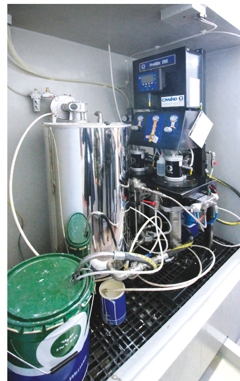
Figure 7: Mascar has chosen the GracoProMix 2KE dosing unit for the primer application stage.
