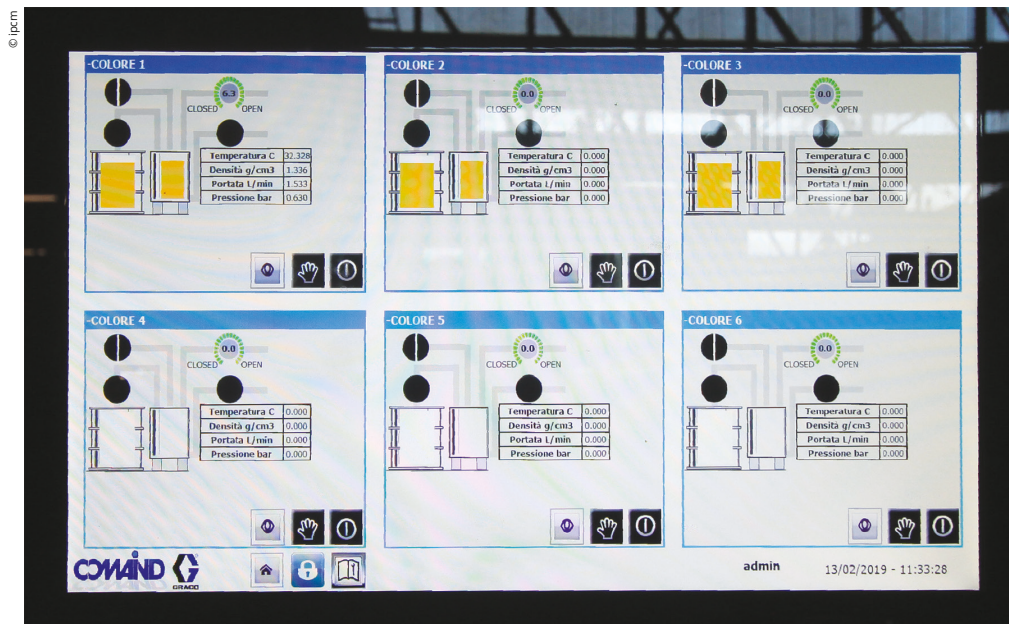
Figures 8 and 9: For the top coat application, Mascar installed the 2KS multi-component dosing system, which allows managing up to five colours but is expandable up to a maximum of thirty.
