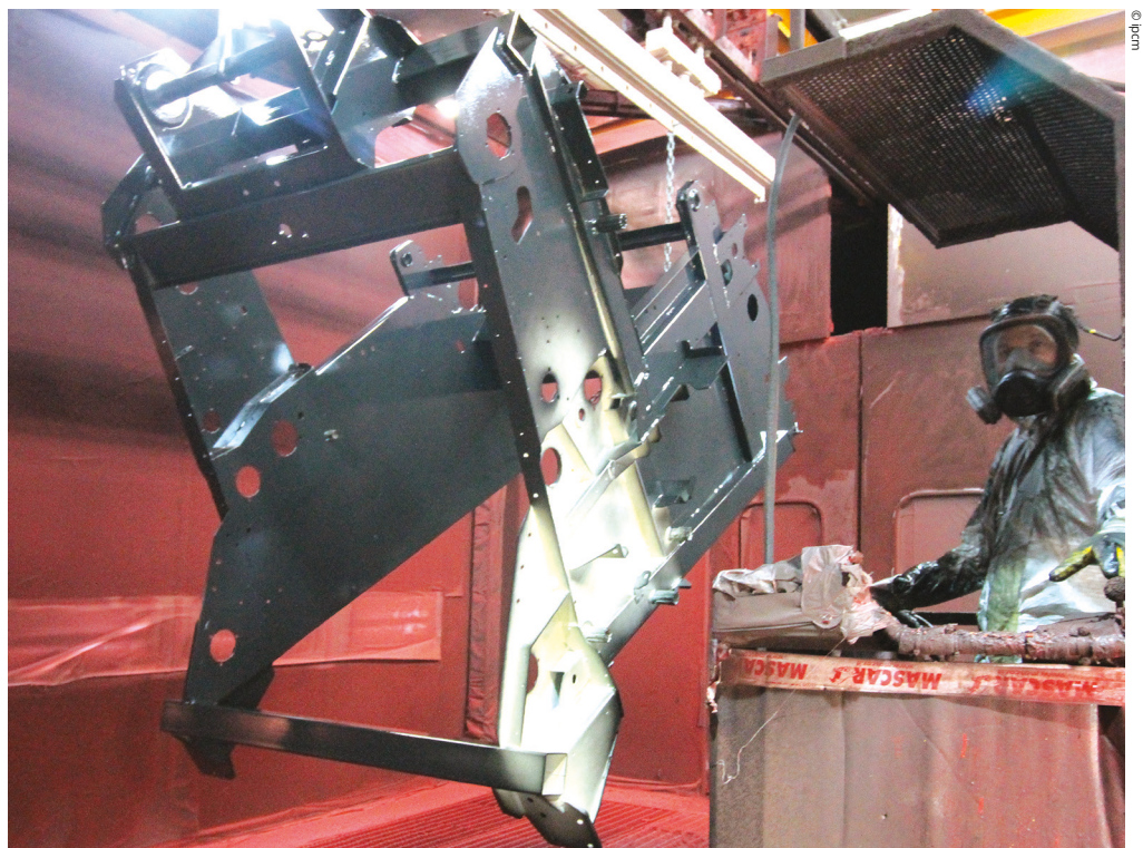
Figure 4: Manual top coat application.
