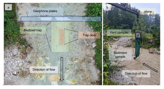
Figure 23: Integrative bedload monitoring at the Johnsbach stream: a) geophone pates and bedload trap (top few), b) vent sampler attached to crane with sediment sample.
