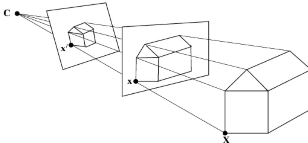
Fig. 8.5. **The cone of rays with vertex the camera centre.** An image is obtained by intersecting this cone with a plane. A ray between a 3-space point  $X$  and the camera centre  $C$  pierces the planes in the image points  $x$  and  $x'$ . All such image points are related by a planar homography,  $x' = Hx$ .
