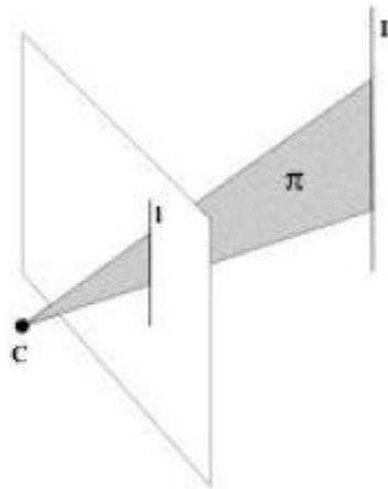
**Fig. 8.2. Line projection.** A line  $L$  in 3-space is imaged as a line  $l$  by a perspective camera. The image line  $l$  is the intersection of the plane  $\pi$ , defined by  $L$  and the camera centre  $C$ , with the image plane. Conversely an image line  $l$  back-projects to a plane  $\pi$  in 3-space. The plane is the "pull-back" of the line.
