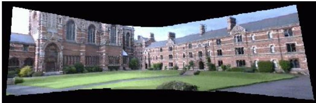
Fig. 8.9. Planar panoramic mosaicing. Eight images (out of thirty) acquired by rotating a camcorder about its centre. The thirty images are registered (automatically) using planar homographies and composed into the single panoramic mosaic shown. Note the characteristic "bow tie" shape resulting from registering to an image at the middle of the sequence.
