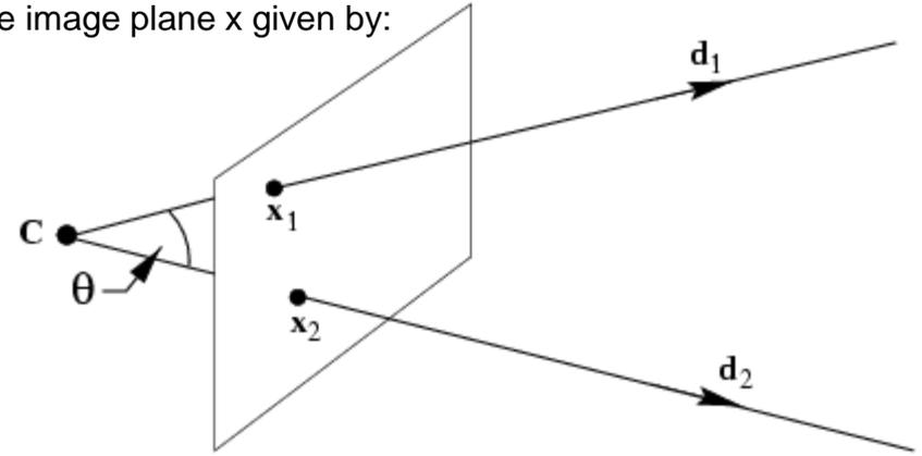
Fig. 8.11. The angle  $\theta$  between two rays.
