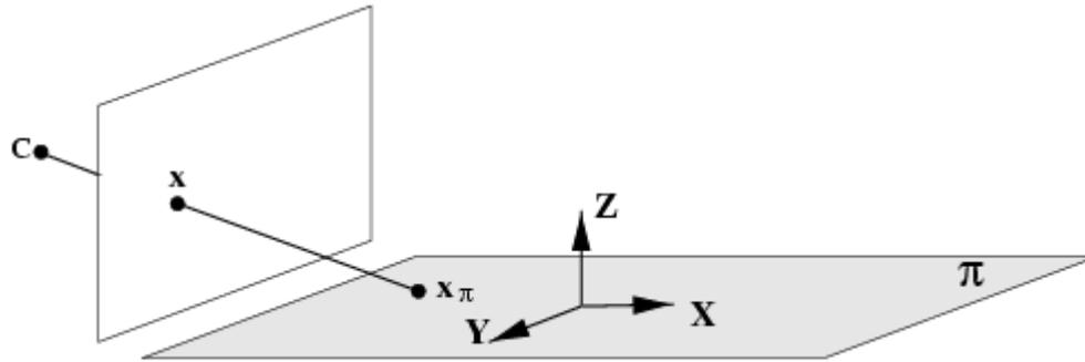
Fig. 8.1. **Perspective image of points on a plane.** *The XY-plane of the world coordinate frame is aligned with the plane  $\pi$ . Points on the image and scene planes are related by a plane projective transformation.*
