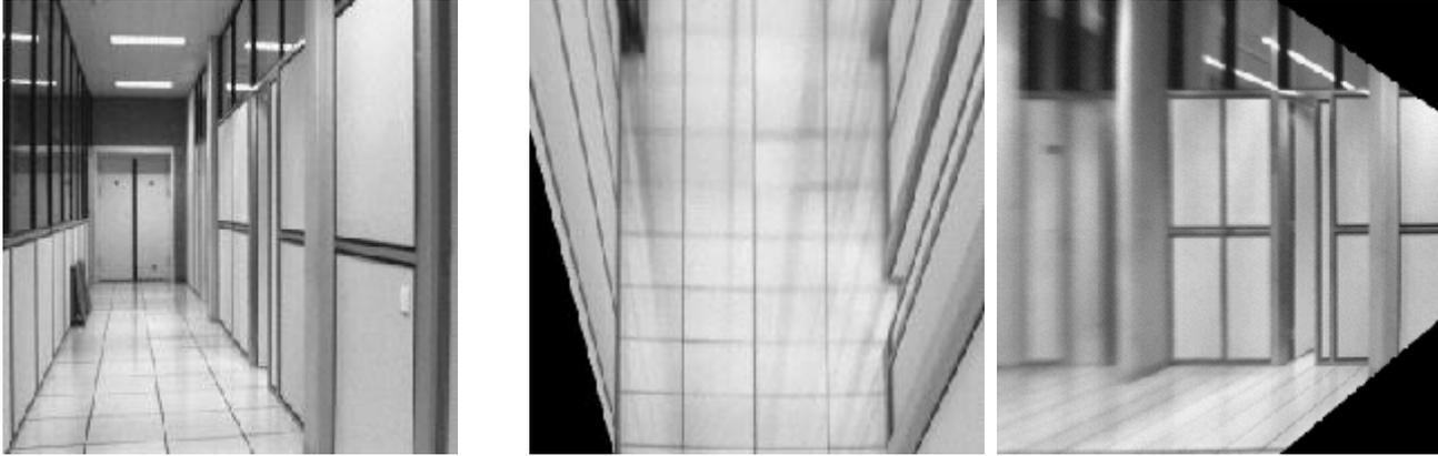
**Fig. 8.7. Synthetic views.** (a) Source image. (b) Fronto-parallel view of the corridor floor generated from (a) using the four corners of a floor tile to compute the homography. (c) Fronto-parallel view of the corridor wall generated from (a) using the four corners of the door frame to compute the homography.
