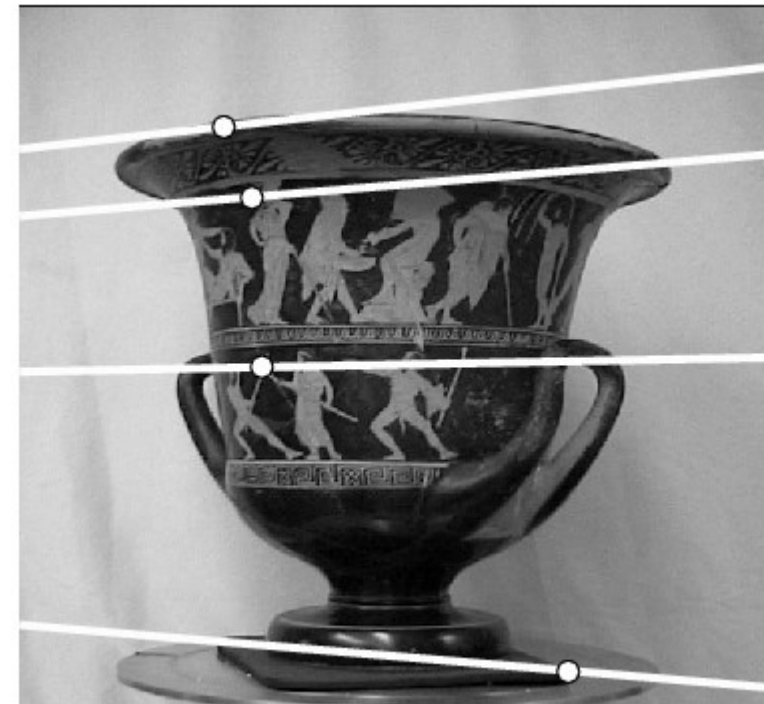
Fig. 9.3. Converging cameras. (a) Epipolar geometry for converging cameras. (b) and (c) A pair of images with superimposed corresponding points and their epipolar lines (in white). The motion between the views is a translation and rotation. In each image, the direction of the other camera may be inferred from the intersection of the pencil of epipolar lines. In this case, both epipoles lie outside of the visible image.
