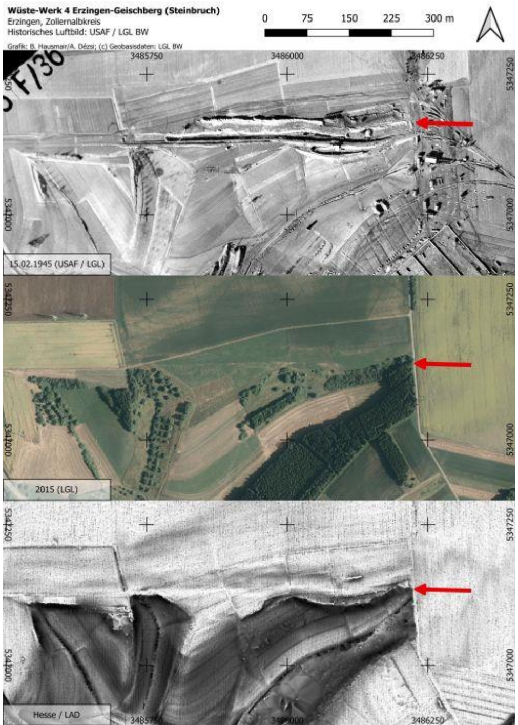
Figure 11: Comparison of historical and modern geodata (orthophoto and digital terrain model) of the site of shale oil factory Wüste 4, Erzingen , showing a persisting large-scale terrain alteration caused by the backfilled quarry (top: photograph: USAAF, 2 February 1945, © KMBD, LGL; middle and bottom: © Geobasisdaten LGL)
