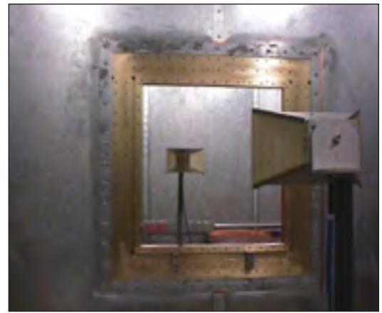
FIGURE 2: Mil-DTL 83528 C test set-up.
