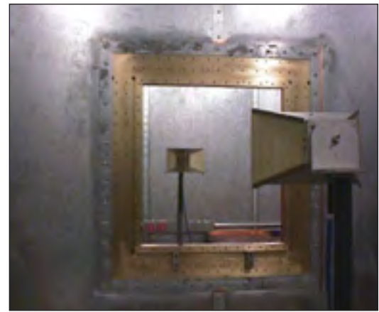
FIGURE 2: Mil-DTL 83528 C test set-up.
