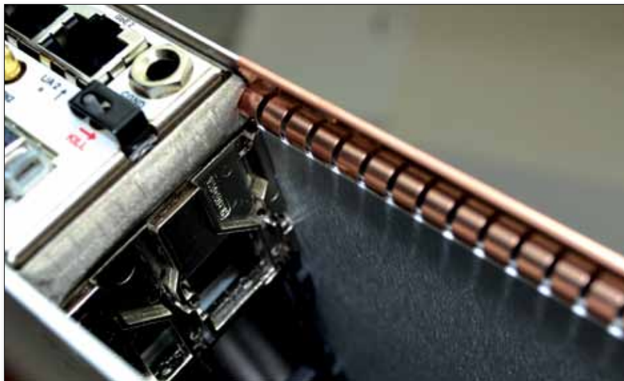
FIGURE 2: Additional gasketing is typically minimal for standard MicroTCA chassis, unless advanced shielding levels are required. The photo shows very standard metal gaskets easily implemented.
