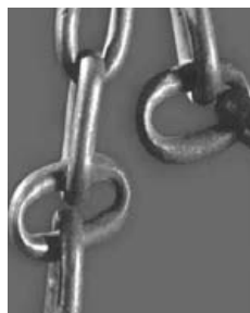
Figure 3 : Inspection for interlink wear can be detected easily by collapsing the chain.
