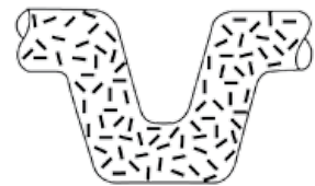
CASTING Random grain flow with larger grain structure makes material weaker than forged products
